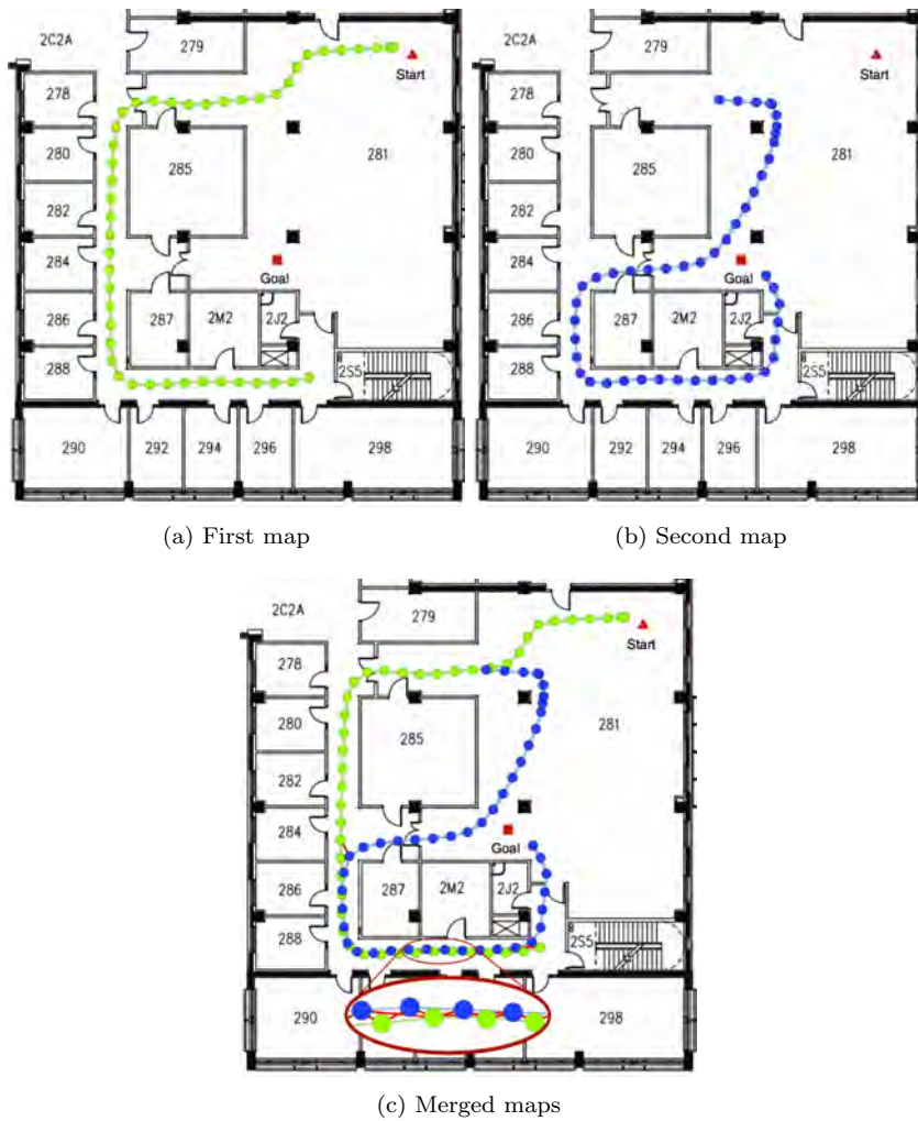
Fig. 6: The top two panels show two appearance-based maps independently built by two robots exploring different parts of the same environment. The last figure shows the merged map and the detail shows some of the edges (red) discovered during the merging process and linking the two maps together.
