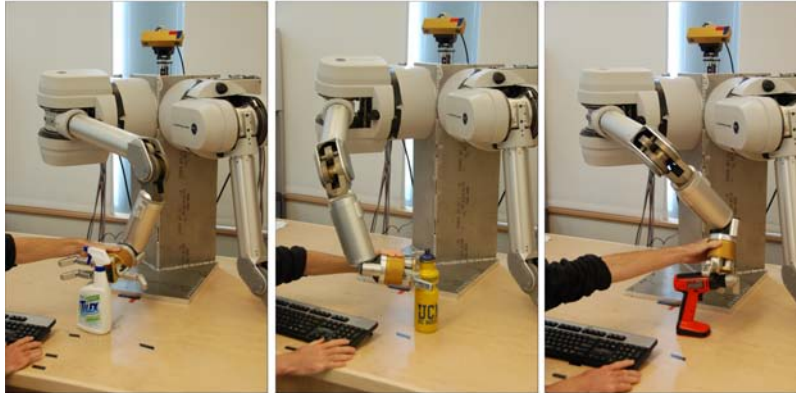
Figure 4.3: A human teaching the robot to grasp a detergent bottle (left), a plastic bottle (center), and a drill (right).
