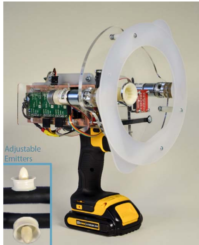
Fig. 1: The Device for Automatic Tuning of Emitters (DATE) can guide workers through fields to adjust passive irrigation emitters. The DATE features a novel two-stage manipulator that cages co-designed adjustable emitters (shown in inset). The handheld DATE and a scaled-down version for robotic manipulators can enable human-robot teams to control irrigation levels at the plant level.
