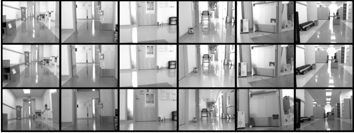
Figure 4.8: With reference to Figure 4.7, the top row shows the images collected by P3AT while building the appearance-based map. Then middle row shows the corresponding view of the P3AT robot upon reaching those waypoints, while the bottom row shows the corresponding views for the iRobot Create.
