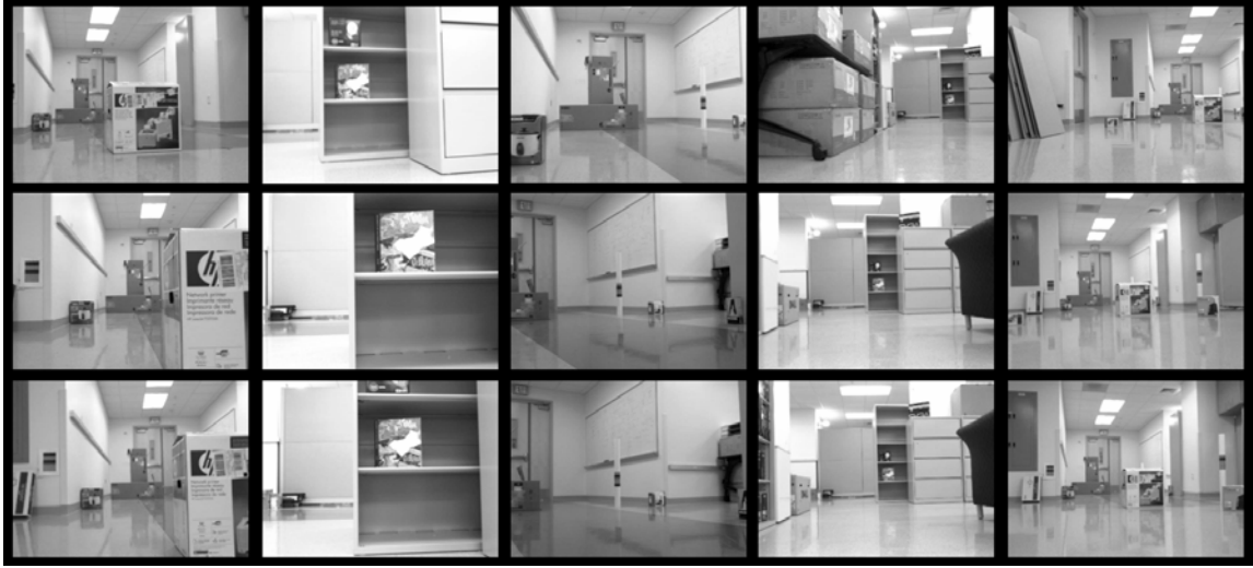
Figure 3.10: Results of the visual navigation algorithm tested on the Create robot. Top row: Initial image taken before starting to navigate. Middle row: Target image captured in an independent run by the Create robot. Bottom row: Final image taken after the navigation algorithm declares that target view is reached.
