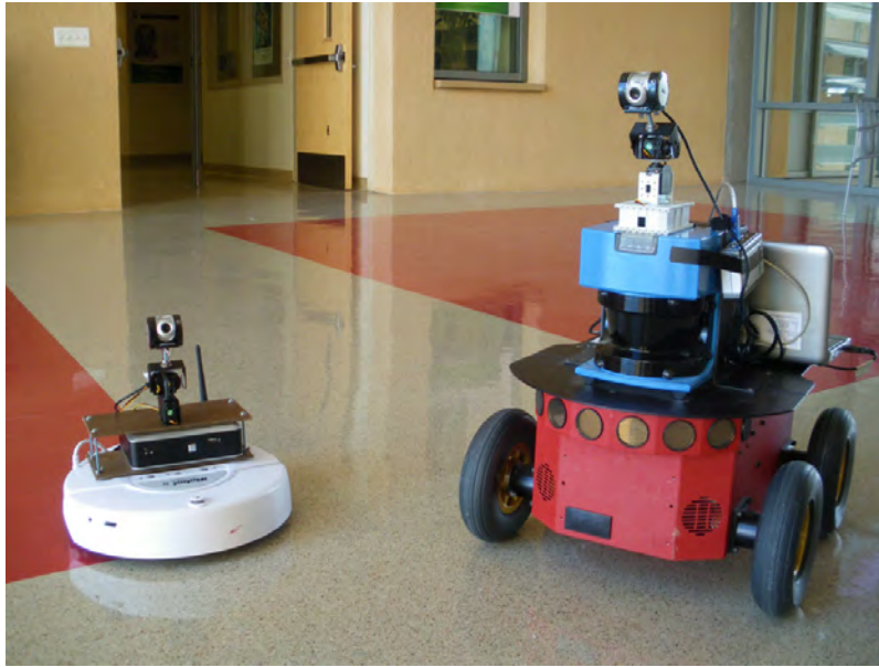
Figure 3.9: The two robots used to test the navigation algorithm in a heterogeneous framework. On the left: an iRobot Create platform; on the right: a P3AT robot.
