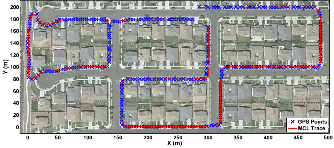
Figure 6.10: Three non-overlapping localized outdoor runs showing the output of the WiFi localizer (line) and GPS receiver (crosses) on top of Google Maps.
