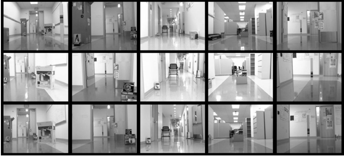
Figure 3.12: The Create robot is navigating towards an image taken by the P3AT robot. Top row: Initial image taken by Create before starting to navigate. Middle row: Target image captured in an independent run by the P3AT robot. Bottom row: Final image taken by Create after it declares that target view is reached.
