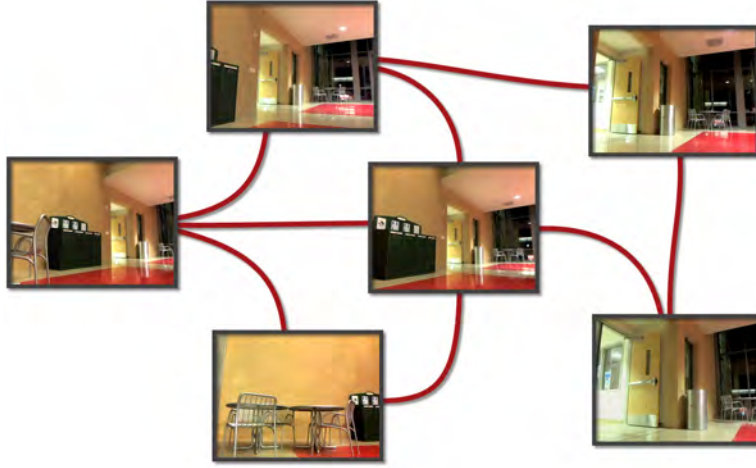
Figure 4.2: A simple appearance-based map with edges inserted between sufficiently similar images.
