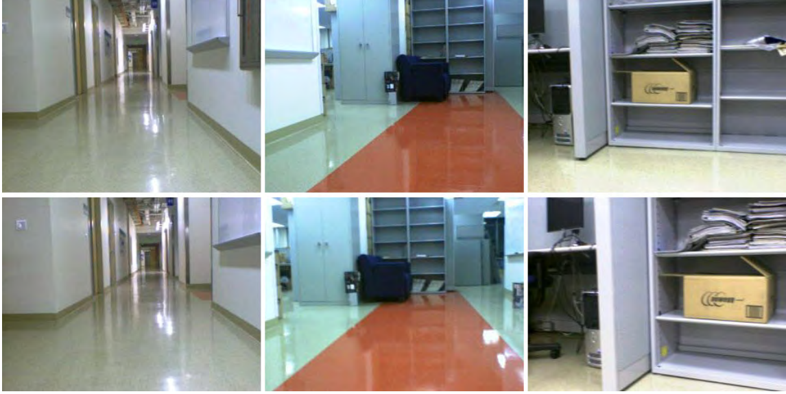
Figure 4.15: Sample image matches are shown. The top row contains query images whereas the retrieved images are shown in the bottom row. Localization accuracy computed for these matches are: 0.052, 0.020, 0.014 (left-right)
