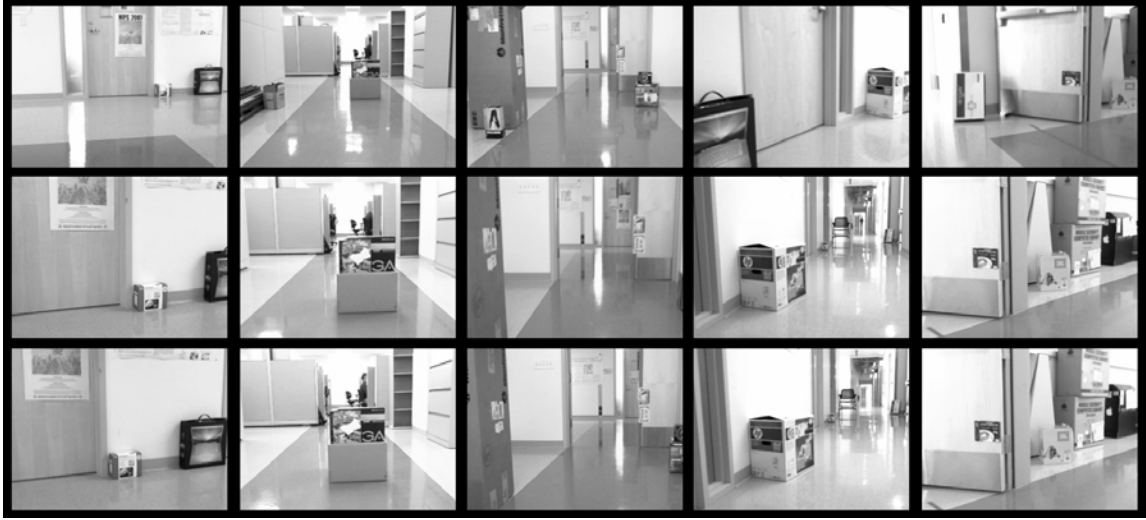
Figure 3.11: Results of the visual navigation algorithm tested on the P3AT robot. Top row: Initial image taken before starting to navigate. Middle row: Target image captured in an independent run by the P3AT robot. Bottom row: Final image taken after the navigation algorithm declares that target view is reached.
