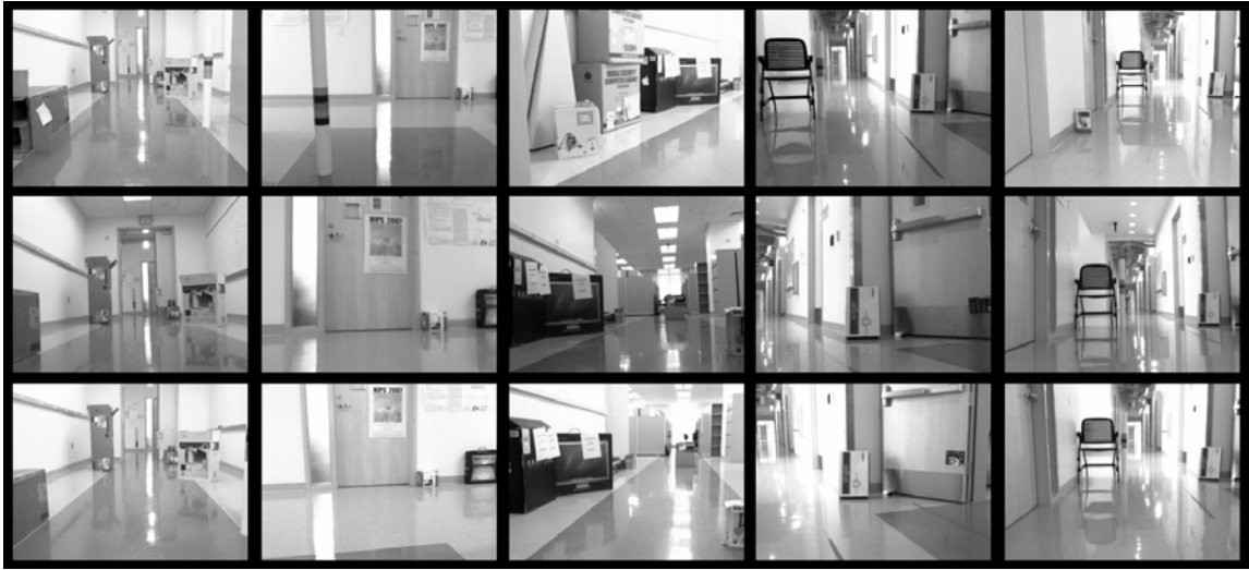
Figure 3.13: The P3AT robot is navigating towards an image taken by the Create robot. Top row: Initial image taken by P3AT before starting to navigate. Middle row: Target image captured in an independent run by the Create robot. Bottom row: Final image taken by P3AT after it declares that target view is reached.
