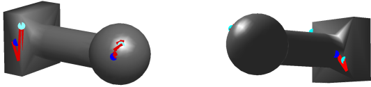
Fig. 6. The figure shows the path followed by three contact points for the testcase joystick (red line). Each contact point starts from the cyan location and end in the blue point. The path is plotted in red.
