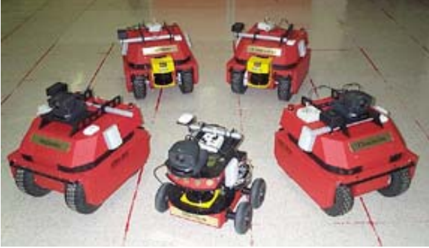
Fig. 2. Heterogeneous Emperor robots used in our experiments. Four of the robots are ATRV-minis, and one robot is a Transit robot.
