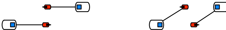
Figure 8: A double tag switch occurring. In this case k = 0 because no robot remains without tags.
