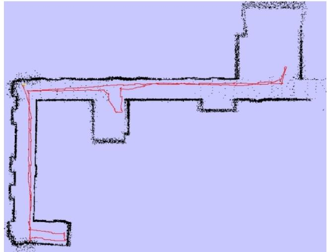
Fig. 10. A map produced by the GMapping algorithm on a data set produced by a simulated P3AT robot.
