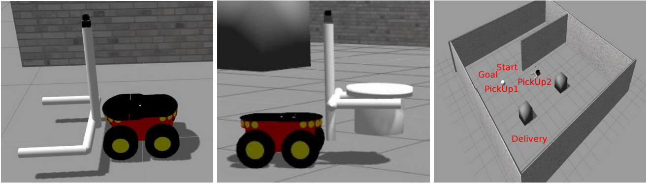
Fig. 2. On leftmost figure, the autonomous vehicle with its gripper fully opened at its lowest position. In the center figure, the vehicle carrying an object. Note that the fork as been closed and lifted. On the right, the environment used for testing.
