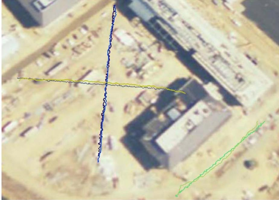
Figure 8: Comparison between the traces produced by the real and simulated GPS sensor. The traces have been superimposed to a satellite image of the University of California, Merced campus.
