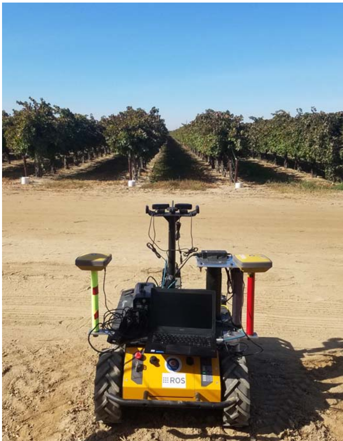
Fig. 1: A test platform for identifying challenges in navigation within a vineyard. Irrigation lines and vine stocks block travel between rows, thus creating motion constraints.
