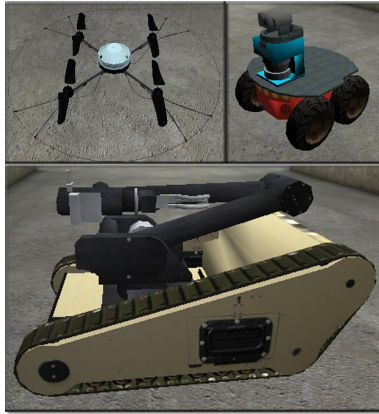
Fig. 1. Simulated pictures of the three robotic platforms used by the UC Merced team. The upper-left screenshot displays the AirRobot, the upper-right screenshot illustrates the P2AT, and the lower screenshot shows the Matilda. As can clearly be seen, the chosen robotic platforms are fervently diverse.
