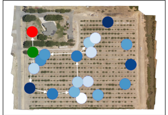
Fig. 3: A test case of size 20 plotted over our test orchard. The white arrows indicate what our GNN-MCTS solved for this problem as the best path.
