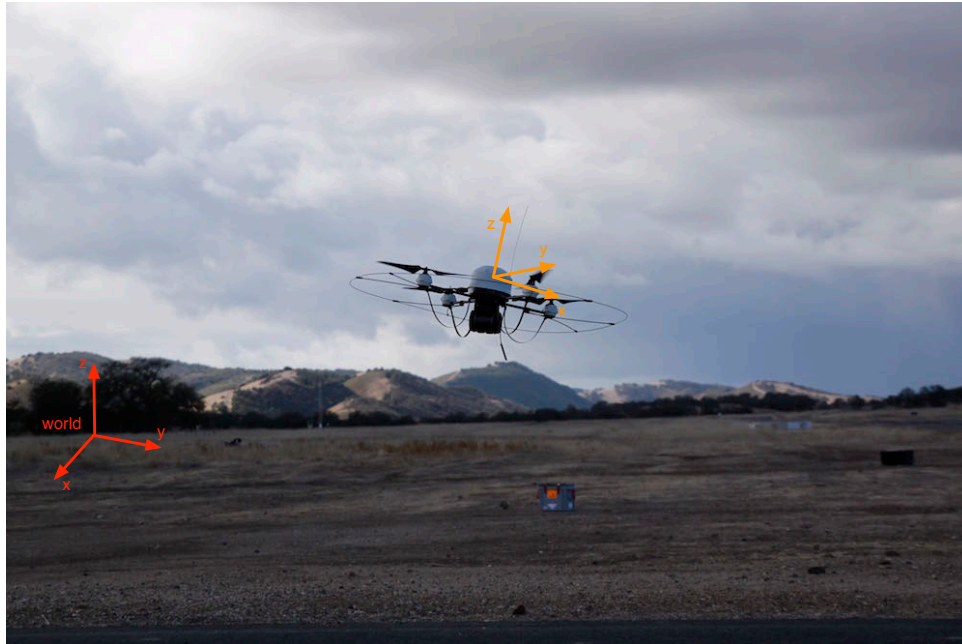
Figure 4.1: The orange frame rigidly attached to the quadrotor defines its pose with respect to the red world frame.
