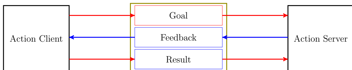
Figure 2.9: Information exchange between client and server in a ROS action. Goal, and results are service calls, while feedback is sent through a topic.
