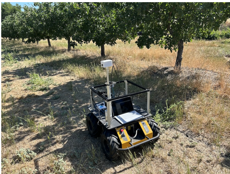
Figure 1.1: A mobile robot collecting thermal images in a pistachio orchard.
