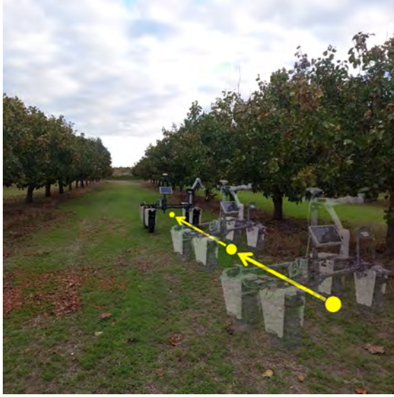
FIGURE 1. A Bonsai's Amiga mobile robot operating in a pistachio orchard showing row-based waypoint movement. While navigating through the waypoints, the robot must remain aware of the spatial variability associated with the canopies of the trees.
