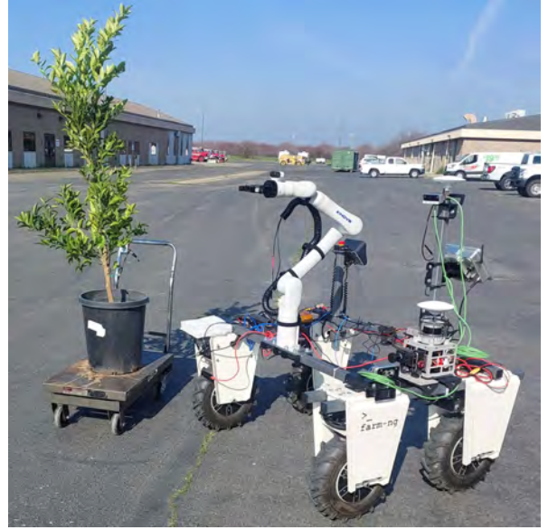
FIGURE 9. Amiga along side our potted citrus plant used in our lab-based experiments.
