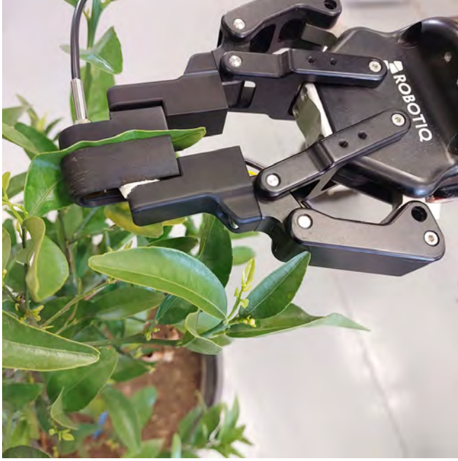
FIGURE 8. The Kinova Kortex with a custom end effector tip on a Robotiq gripper grasping a citrus leaf during a lab experiment.
