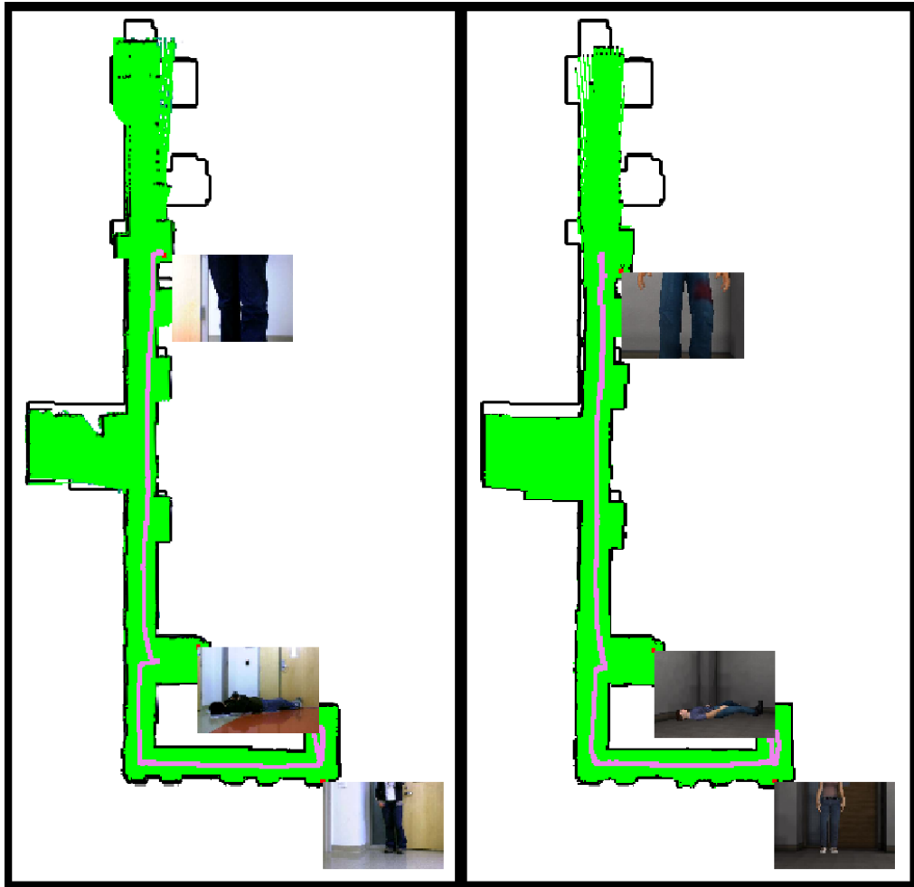
Figure 7: This figure shows the composite map generated by the real platform (left) and the simulated platform (right). The attribute overlay is not displayed.
