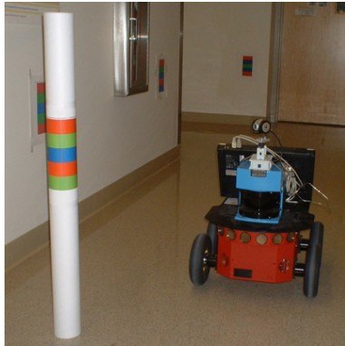
Figure 8: The robotic platform used to validate the proposed algorithm. On the left one marker used for localization is visible.
