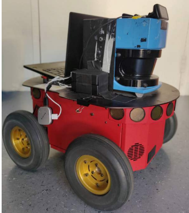
Figure 7.7: Pioneer Robot 3AT mounted with a Laptop, a LIDAR, a RGB camera and two IMU um7.
