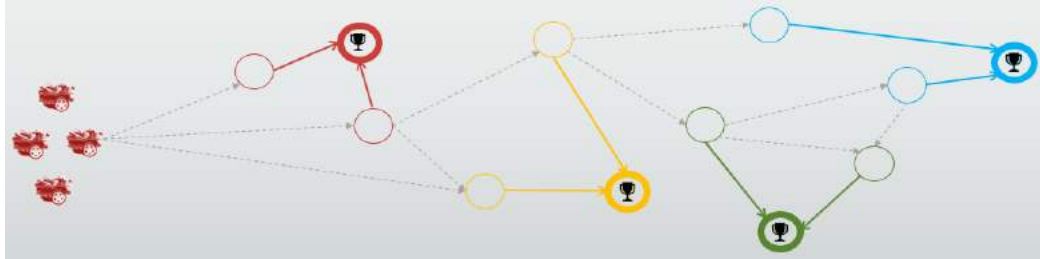
Figure 2.4: Rapid Deployment Problem with a group of robots trying to reach different targets with multiple observation points.
