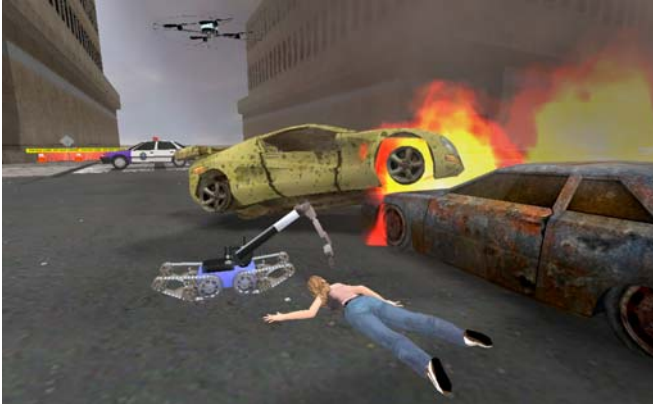
Figure 1: USARsim is the simulation engine used to run the RobocupRescue Virtual Robots competition. The picture shows one of the environments used during Robocup 2006. A tracked Telemax robot and a flying Air-Robot platform can be seen in the screenshot.
