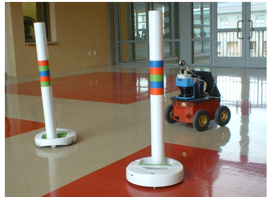
Fig. 1. The robot used for the experimental validation. Two iRobot Create platforms acting as static landmarks can be seen. Visual landmarks can be observed on the poles mounted on the stationary robots.
