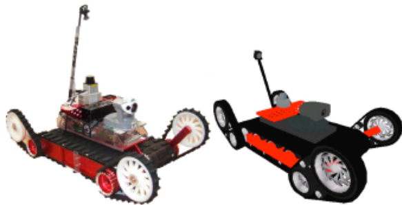
Figure 2 On the left, the Kenaf robot, a USAR platform developed at the Tohoku University, Japan. On the right, the simulated model inside USARSim. The model was contributed by the same group that developed the real robot.
