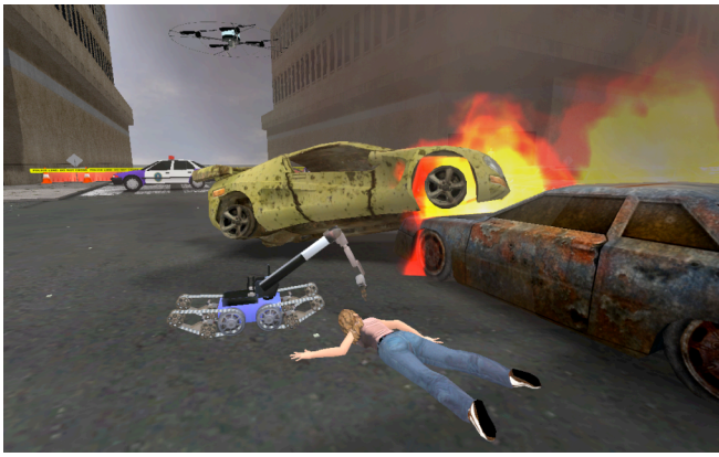
Figure 6: USARSim is the simulation engine used to run the RobocupRescue Virtual Robots competition. The picture shows one of the environments used during Robocup 2006. A tracked Telex robot and a flying AirRobot platform can be seen in the screenshot.
