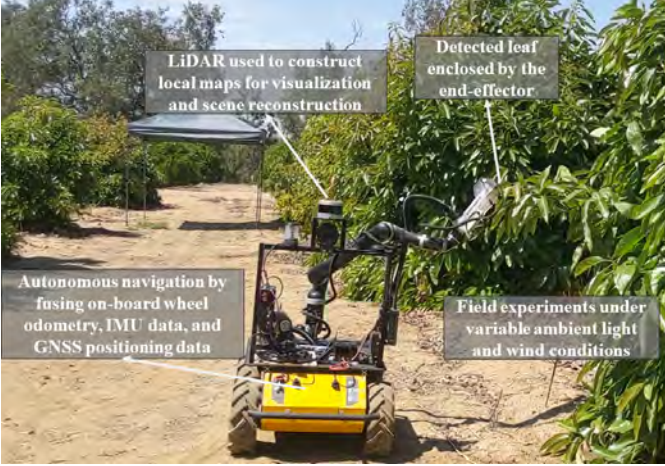
Fig. 3: The agricultural robot used in this work for robotic assessment of a crop’s need for watering.
