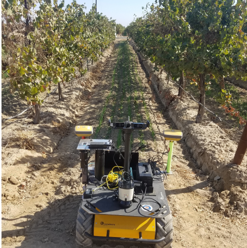
Figure 2.1: The Husky robot has been retrofit with a soil moisture sensor that can be inserted in the soil to collect data (the soil moisture probe is visible on the left).
