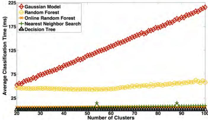
**Fig. 8** Average time, in milliseconds, it takes to classify 10 observations, as the number of clusters increases during robot exploration. The Gaussian Process and Support Vector Machine algorithms are omitted because they take too much time relative to the other algorithms (i.e., 3.05 and 9.07 seconds, on average, for a map size of 100 clusters).
