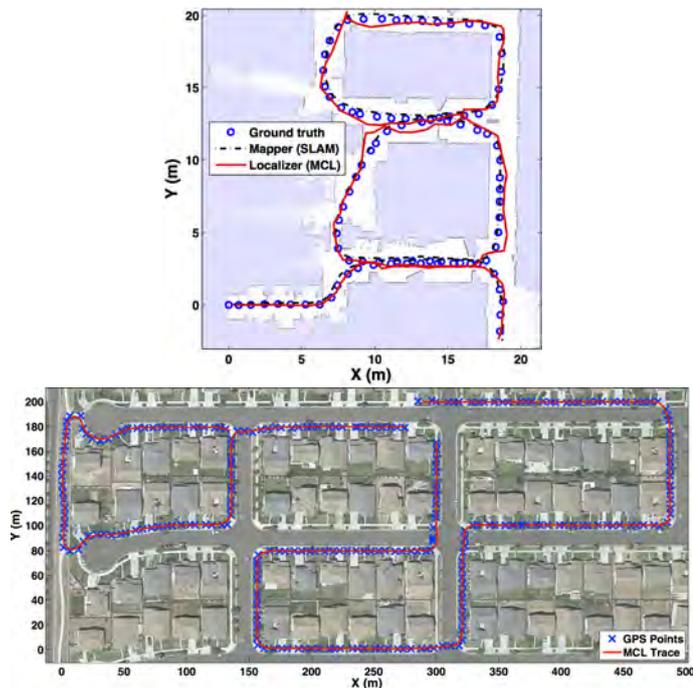
**Fig. 9** Experimental results for indoor (top) and outdoor (bottom) scenarios, showing the results of our WiFi localization (red) against ground truth (blue) and SLAM (black, indoor only). For the outdoor scenario, GPS is used as “ground truth”.
