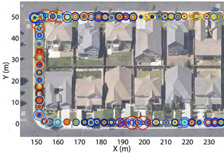
**Fig. 1** Illustrative representation of the WiFi readings in an outdoor environment, superimposed on Google Maps. The size of each ring is proportional to the AP's signal strength and each color represents a unique AP. The Cartesian coordinates are derived from a GPS sensor.
