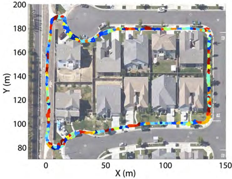
**Fig. 2** Illustrative representation of the clustering algorithm in an outdoor environment, superimposed on Google Map. The different clusters are represented by different colors and each encompass a varying number of WiFi observations.
